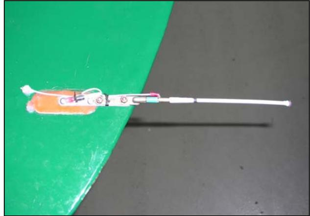
**Figure 6: Instrumented Static Wick**
